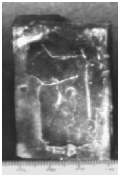
Fig. 3. Ceramic part fired under the same time/temperature conditions outside of the partially isostatic debinding system.
